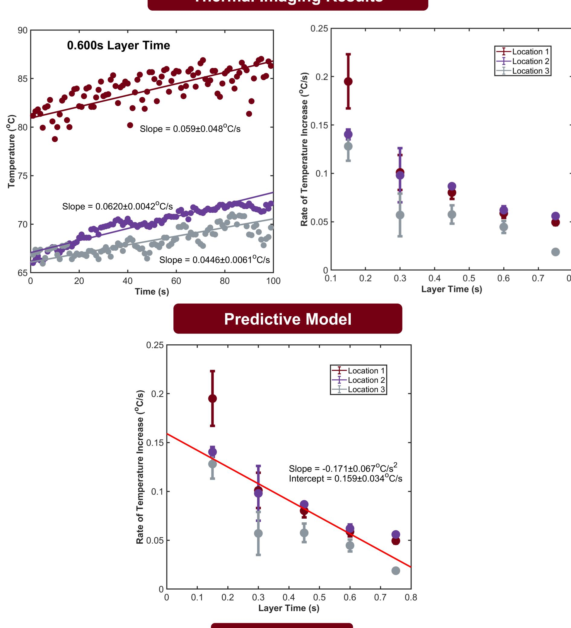
The temperature of Photopolymer Resin increases linearly for the duration of a print.
